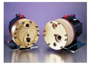
Hydra-Cell H/G-25 pumps are used for spraying cyanide solution over gold ore and then pumping the recycled solution. Metallic head models have a maximum flow rate of 20 gpm (75.7 l/min) and pressure rating of 1000 psi (69 bar).
