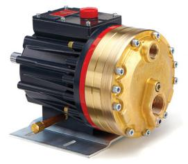
Pump Model: H25XKBTHFEHA with Oil Level Monitor Mounting Kit 103-000 & 103-010 Flow Rate: 15 gpm (57 l/min) @ 800 rpm Pressure: 700 psi (48 Bar) Application: Pumping seal flush water to slurry pumps
